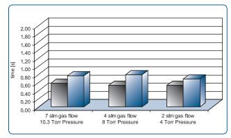
Figure 1 — SmartPower<sup>®</sup> System Performance SmartPower system performance with 50%  $NH_3$  / 50%  $N_2$  plasma at 3 kW
