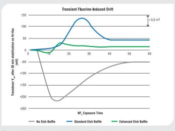
Figure 4 - Validation data for the effect of fluorine absorption on capacitance manometer drift and for the impact of different etch baffle designs
