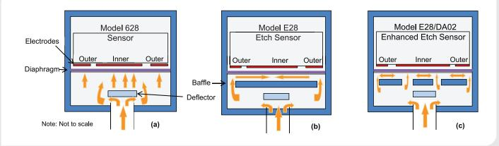
Figure 3 - Manometer baffle evolution
